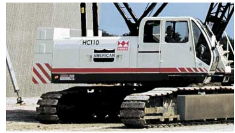
Hydraulic removable counterweight system
